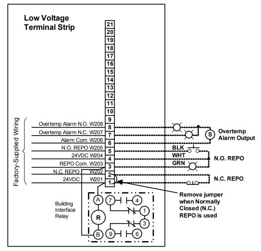
Figure 15 Typical control wiring for units without monitoring
